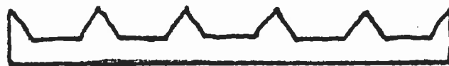
Figure 16. The Stoler frame spacer is a specially cut strip of metal which attaches to the rabbets (shelves) of the brood chamber and honey supers.
